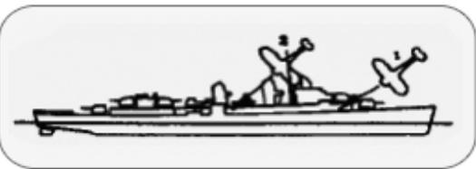
From the battle damage report dated 1945. Japanese suicide plane carrying bomb crashed into No. 2 handling room from ahead. Bomb detonated in wardroom. Serious damage to bridge. Serious fire in No.2 handling room. Almost simultaneously second plane carrying bomb crashed at about frame 100. Bomb blew No.2 smoke pipe clear of ship and demolished superstructure from after part of galley to torpedo workshop. Serious fire in sick bay.
