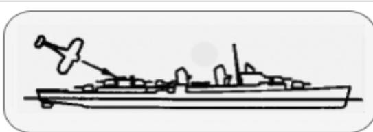
From the battle damage report dated 1945. Japanese suicide plane carrying bomb crashed into 40mm gun No.5. Bomb detonated, demolishing deck house between 5-inch guns No.3 and 4. Minor fire extinguished in 5 minutes. Main deck buckled but not ruptured. 5-inch guns No.3 and 4 severely damaged.
